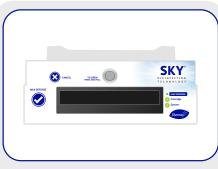
**Step 8 -** After thirty (30) seconds, the system warm up process will be completed. The System LED light will be solid green. Additionally, the
