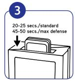
Once the rollers engage, the unit will begin disinfecting the device - it will take 20-25 seconds for standard mode, and 45-50 seconds for max defense mode.
